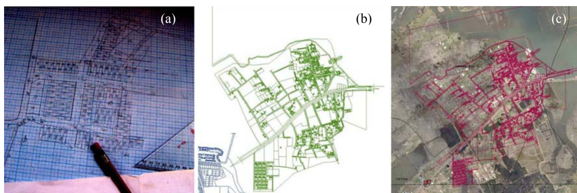
Figure 3: (a) Creation of a simple community based land ownership map (part of); (b) CBM converted to AutoCAD to record land ownership agreement and details; (c) CBM rectified using orthorectified aerial photography.
